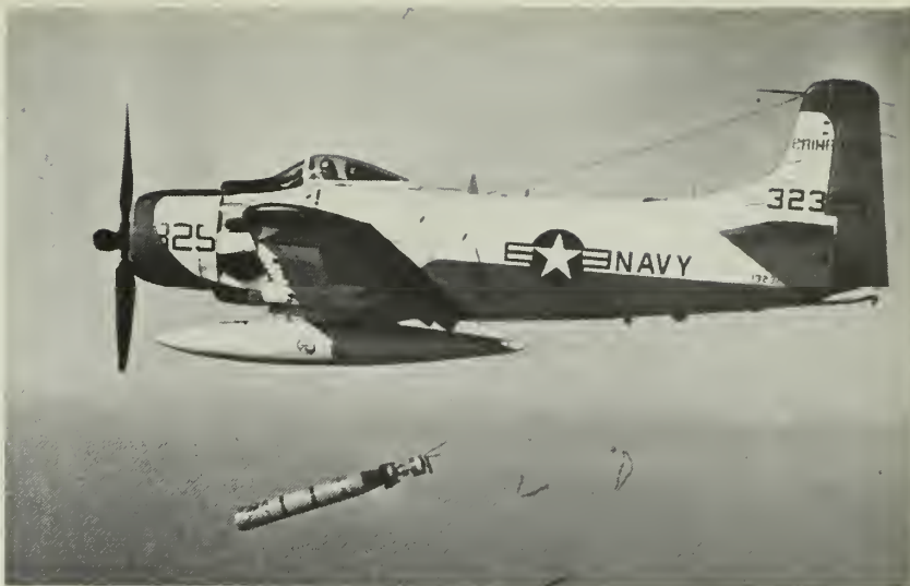
PARACHUTE TORPEDO—Mark 44 torpedo is a new lightweight ASW weapon that seeks out target. It can be dropped by plane or fired from shipboard.
